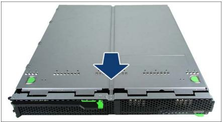
Figure 16: Closing the server blade
